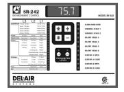
The SR-242's faceplate features a LED Status window, 1 parameter list, 1 outputs list with 11 LEDs, 2 function buttons (L2 and L3), 2 parameter buttons (▶ and ▶) and 2 value setting buttons (▶ and ►). Below is a brief description of all features, from left to right on the faceplate.
