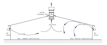
The W3 works with an actuator or winch to pull open and closed. Between 35 & 50% baffle opening, the air is directed upward. At this stage, the bottom edge of the baffle remains sealed, preventing air from escaping horizontally. From 50 to 100% opening, the air is allowed to flow across the facility providing cooling benefits.
